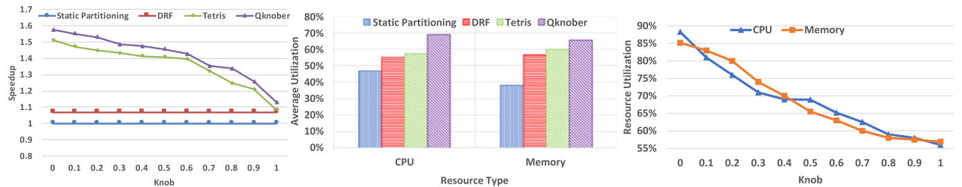
Fig. 7. The comparison results of performance and resource utilization for Static Partitioning (i.e., non-sharing case), DRF, Tetris and QKnobler under different knob configurations, where the speedup of makespan is computed over that of Static Partitioning.
